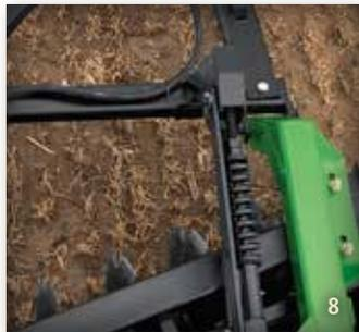
(11) The over-center locking wing design on 21- to 22-foot offset disks prevents wings from flexing up during operation.
