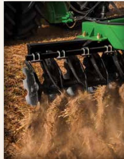
Frontier Tandem Disks give you the options of 309 to 370 pounds per blade; a 9-inch cutting depth; 10 1/2-inch blade spacing; and blade diameters of 26 and 28 inches.
