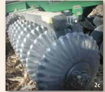
(3) Fully adjustable blade scrapers reduce wear in light, dry soil and keep you going even in wet, sticky soil.
