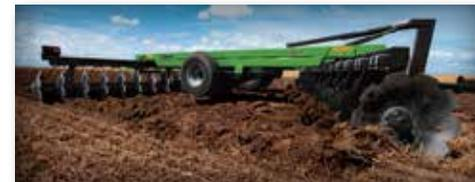
Frontier Heavy Offset Disks offer the right balance of weight-per-blade, penetration depth, blade spacing, and blade diameter for any soil condition.
