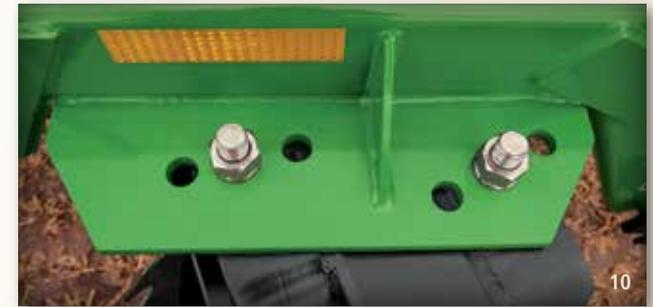
(10) The simple bolt adjustment allows the gang angle to be more aggressive in heavy residue or less aggressive in lighter soils on offset disks.
