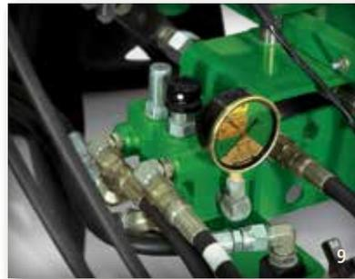
(9) Hydraulic wing control valve allows varying hydraulic pressure to the wing-fold cylinders, which transfers weight from the mainframe to the wings for improved penetration in hard ground or heavy soil.
