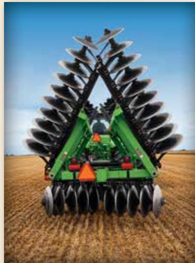
Disks are designed to provide maximum field coverage with each pass, yet convert to a narrow profile for easy transport. Dual folding cylinders allow both sides of the frame to hydraulically fold over to create a narrow transport width.
