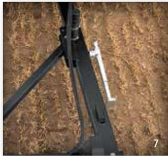
(8) Protect disk blades during transport with the leveling linkage. In the field, it also promotes stability over rough terrain for a smooth, consistent soil profile. Available on Heavy Offset Disk only.
