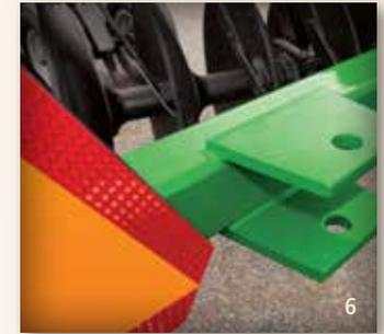
(7) A sturdy, adjustable level-lift hitch makes sure weight stays on disk blades, where it does the most good. Plus, this design lets you make short, tight turns while maintaining excellent blade penetration.
