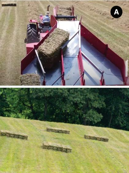
The Norden Hay Accumulator uses gravity and a simple mechanical system to efficiently arrange bales into a group that is then dropped in the field. A Norden Mfg Grabber or Tie-Grabber mounted on a front end loader or skid steer picks up the bales to load them onto a waiting truck, trailer or wagon. The groups can then be unloaded into the barn via the grabber without an operator ever needing to touch a bale.
